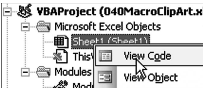
Figure 112. The code to intercept the hyperlink has to be on the code pane for the worksheet.
