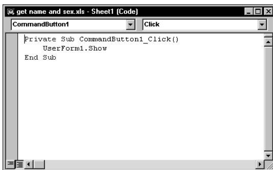
Figure 13-8: The CommandButton1_Click procedure is executed when the button on the worksheet is clicked.
