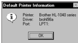
Figure 11-15: Getting information about the active printer using a Windows API call
