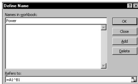
Figure 3-4: You can name a formula that doesn't appear in any worksheet cell.
