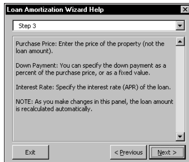
Figure 25-7: User help is presented in a UserForm that copies text stored in a worksheet.
