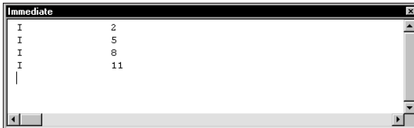
Figure 10-6: Using the Immediate window to display results while a function is running
