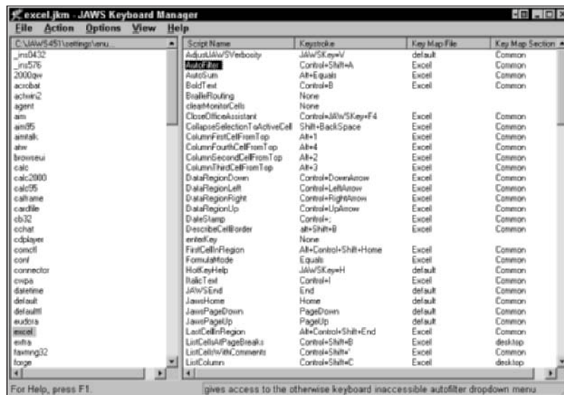
Figure 13-3: The Keyboard Manager allows you to define, for any application, new keystroke sequences and associate them with scripts that can be run by JAWS.
