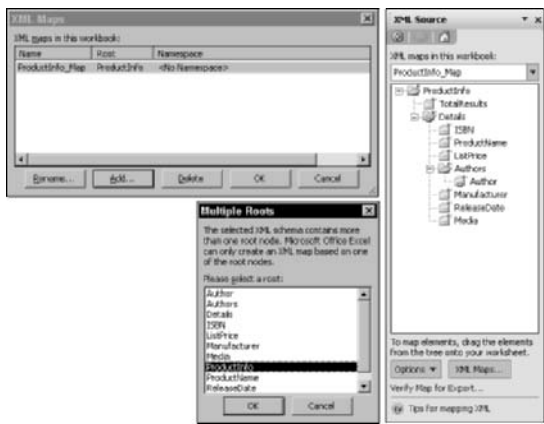
Figure 12-14: Creating an XML Map directly from a Schema (XSD) file
