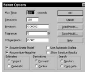
Figure 8-14: Remember to check the boxes of the Assume Linear Model and Assume Non-Negative options when performing linear programming optimizations.
