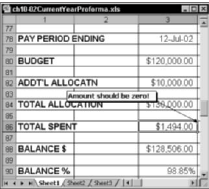
Figure 10-14: Appearance of a ghost: The total spent at start of year should be zero, but $1,494 is already reported to have been spent!
