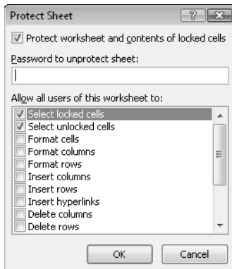
Figure 6-5: Using the Protect Sheet dialog box to specify what users can and can't do.
