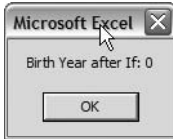
Figure 7-9. The iReturn variable did not fall into the If...End If statement, and it is still incorrect.
